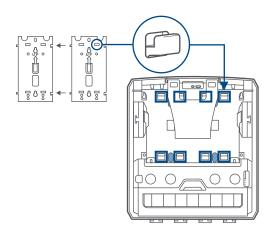
**Direct Mount:** Position unit on wall so that the top is level. Use key to open front cover and mark screw locations where indicated with circles. Secure unit to wall with four anchored screws appropriate to the type of wall in locations previously marked.
