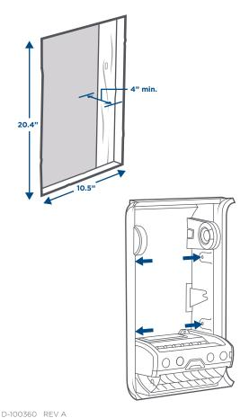
**Mounting:** A hole 20.4" x 10.5" must be cut into your wall to accommodate this dispenser. Before cutting your hole be sure to consider stud location inside the wall so that the dispenser can be inserted without obstruction.
