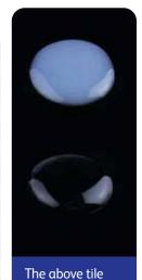
has 5 coats of floor finish. The top half shows immediate softening of the finish, as indicated by the whitening effect, caused by a high alkaline (11 pH) disinfectant. The bottom half shows that the Virex®II 256 product has no effect, αs evidenced by the absence of any whitening.
