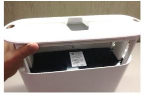
(3) Push down on one end of the black platform and separate the platform tabs from the cartridge tracks (as shown).
