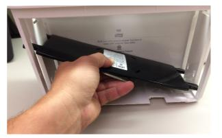
(10) Place the cartridge into the cassette and position it so it is about halfway down. Angle the platform so the tabs get below the green level indicator on one side.
