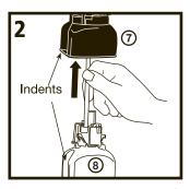
Feed dispenser straw on the refill bottle (8) up through the bottle support (7) and dispenser assembly (1), aligning the two indents in the bottle and the support. Slide the bottle upward until it snaps into place.
