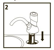
Position the dispenser assembly by guiding the threaded stem through the hole in the counter. Make sure the spout is facing into the sink bowl. Press down firmly on dispenser assembly to ensure it is securely attached to counter.
