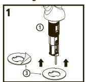
Locate the adhesive gasket ③. Remove the liner from the top of the adhesive gasket and thread it onto the stem of the dispenser assembly ① to affix to to the bottom of the dispenser. Remove the liner from the bottom of the gasket.
