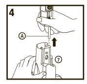
Align the metal rod (A) from threaded stem with small guide hole in the bottle support (7). Slide the bottle support up onto the rod.
