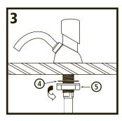
From underneath the counter, secure lock washer (a) and mounting nut (b) and tighten to underside of counter.
