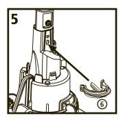
Secure the bottle support to the dispenser assembly by pushing the retaining dip (a) into place.
