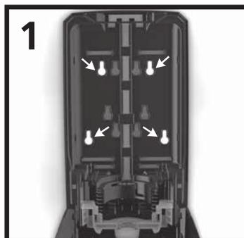
1 Using back plate as template, mark and drill center holes in wall using 1/4" (6.3 mm) spiral masonry drill bit or 1/4" (6.3 mm) wood drill bit. **Recommended holes shown.**
