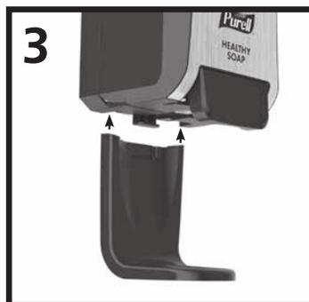
3 Install the SHIELD™ Floor and Wall Protector into the bottom of the dispenser by aligning plastic tabs on the SHIELD with slots on the dispenser and sliding up until the tabs snap into place. (SHIELD is included with Sanitizer Systems and can be ordered for Soap Systems).
