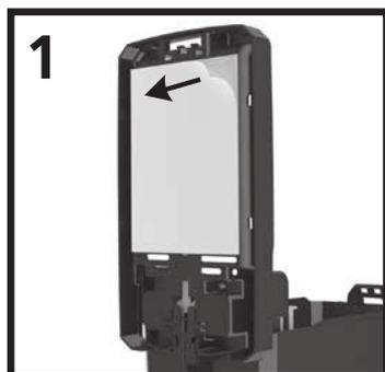
1 Clean installation surface with an alcohol pad. Allow surface to dry for 60 seconds, then peel paper off installation tape and press firmly against installation surface for 30 seconds. For maximum adhesion, wait 24 hours before loading refill or using dispenser.
