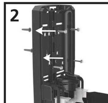
2 Install #10 x 1" (2.54 cm) anchors into drilled holes, flush against surface. Insert type A #10 x 1" (2.54 cm) fasteners into 4 installation holes in back plate, through installation tape. Tighten fasteners securely. **Be careful not to over-tighten.**
