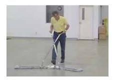
Pull handles outward to expand V-Sweeper panels for wide area cleaning.
