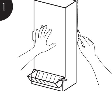
Position dispenser in the selected area on the wall. Mark the desired top and each side as a guide for bracket placement and set the dispenser aside.
