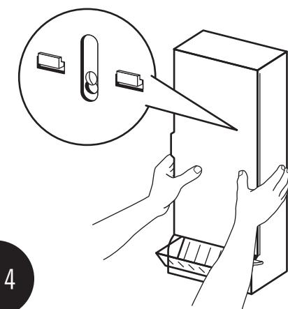
Attach dispenser to bracket by slipping over corresponding openings until it is secured in place.
