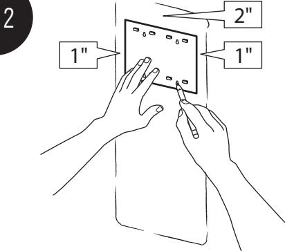
Line up the bracket within outer markings as follows and mark position through screw holes.
